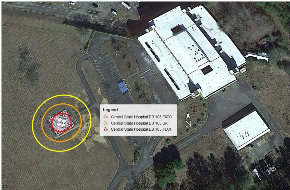
Figure 2-5: Vertiport Landing Dimension Overlay
