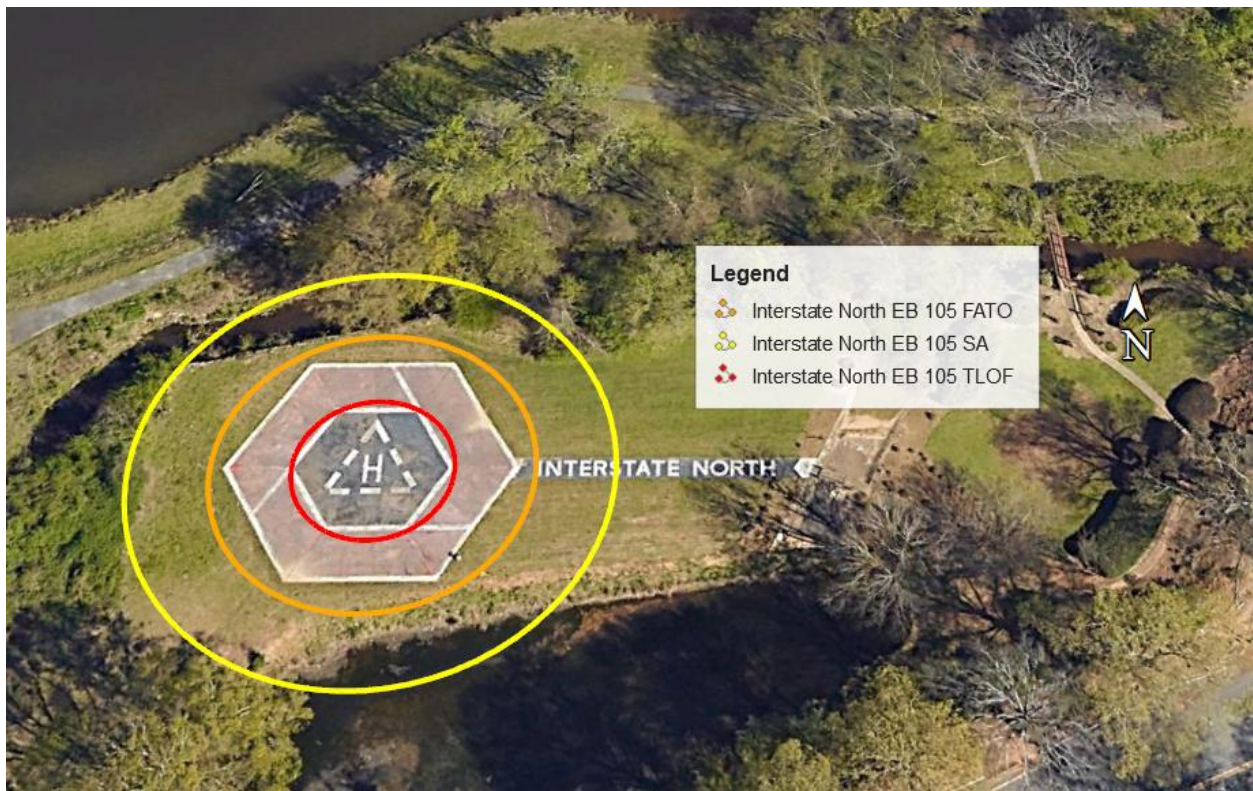
Figure 2-11: Vertiport Landing Dimension Overlay
