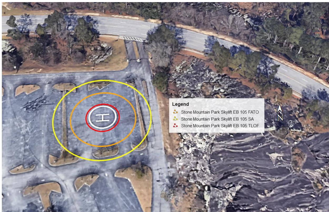
Figure 2-26: Vertiport Landing Dimension Overlay
