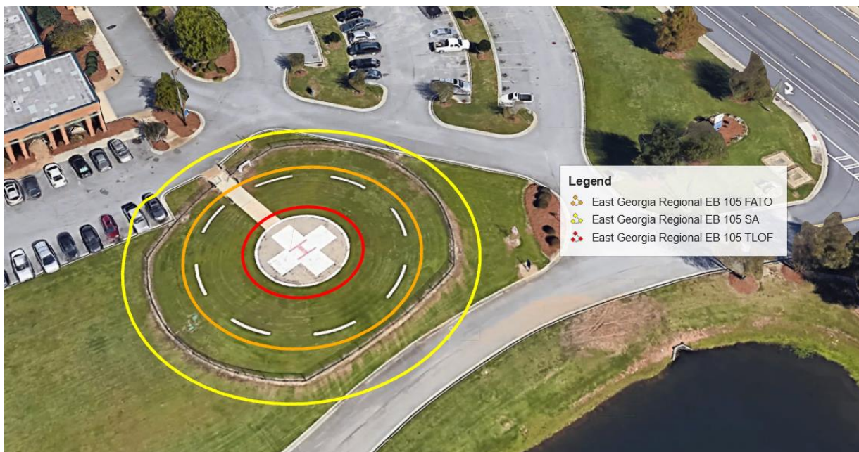
Figure 2-8: Vertiport Landing Dimension Overlay
