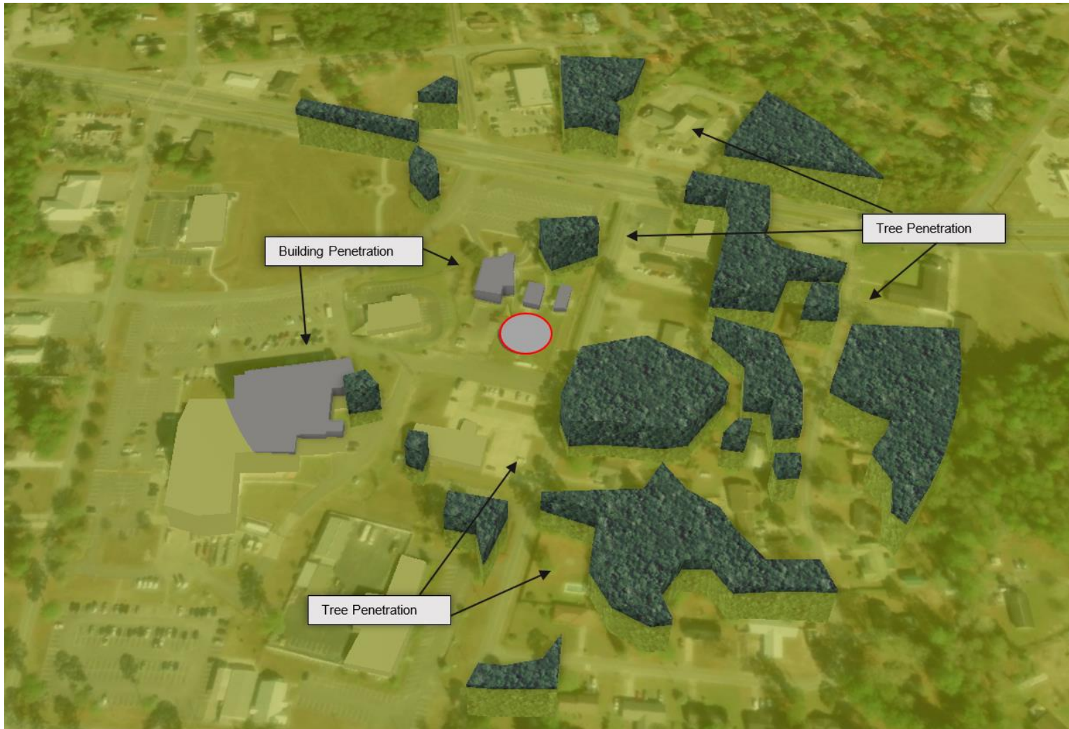
Figure 2-32: 39GA Site and Cone Penetrations
